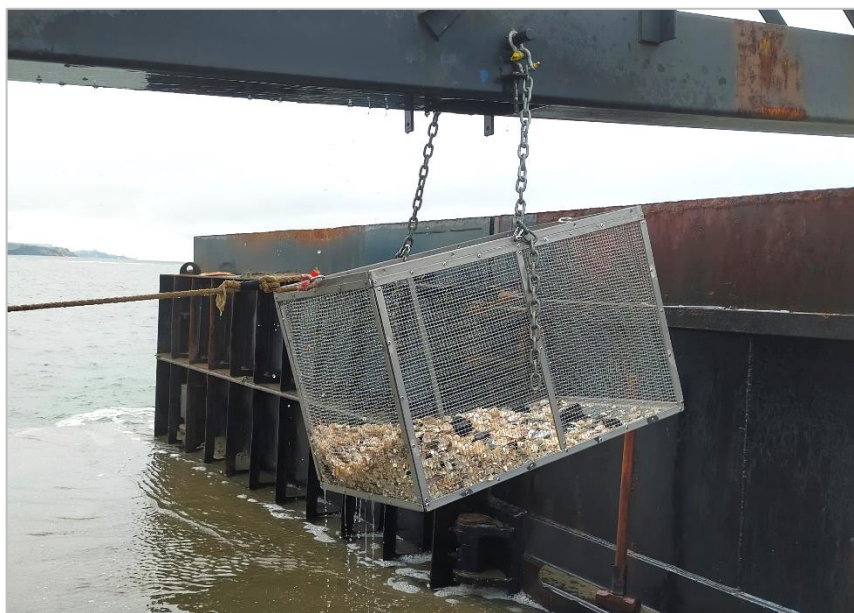
Figure 2-2: The 9 mm sieve basket placed under an outlet in the discharge chute, sampling 6 m 2 of seabed.
