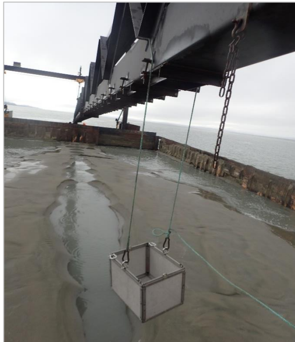
Figure 2-3: The 1 mm sieve basket that collects the sediment surface sample from the first discharge chute opening. Sand collection hopper on Kaipara Karrier VI in the background.
